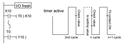
◆ From above diagram, if the timer contact position put before timer coil, then the bad accuracy is "+2t".
